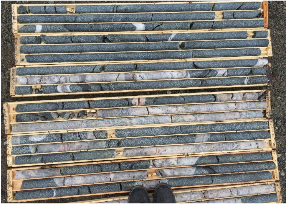
Photo 1. Photo highlighting pegmatite dykes, often spodumene-bearing, in hole WL17-07 showing core from 2.6 m to 30.5 m downhole.
